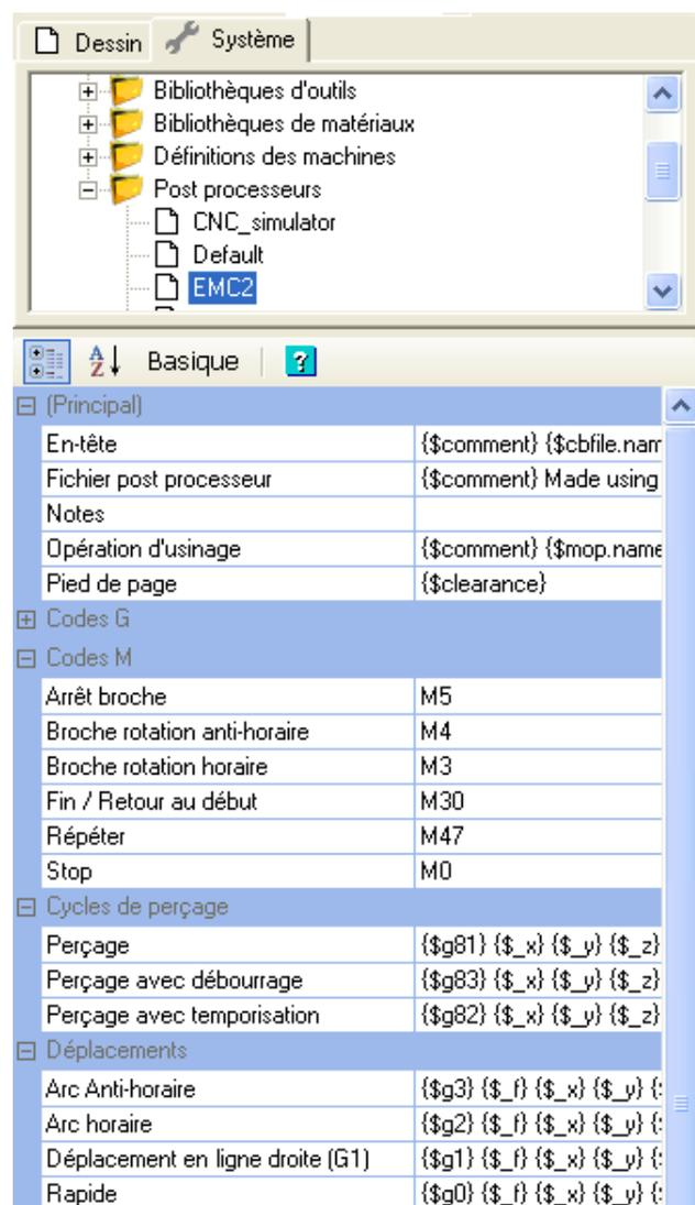
The screenshot shows the 'Système' tab in CamBam. The left pane shows a tree view with 'Post processeurs' expanded, listing 'CNC\_simulator', 'Default', and 'EMC2'. The right pane shows a table of G and M codes with their corresponding G-code commands.
